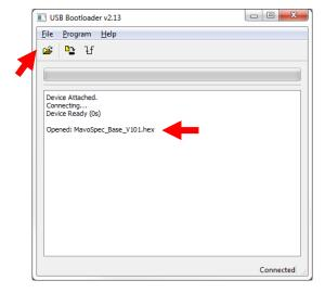
Start the firmware update by clicking the button and wait until the program has completed all installation steps (erasing, writing and verifying). This takes about one minute.
