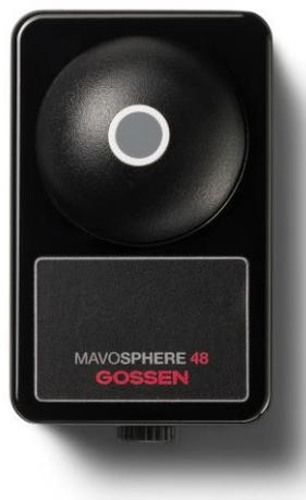
The set includes the sphere in housing with a coder for automatic detection of the accessory. It is delivered with the certificate of factory absolute spectral calibration.
