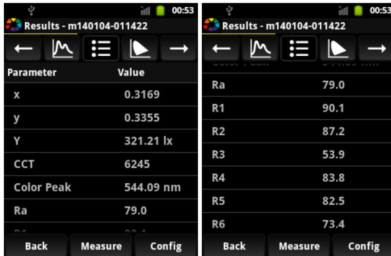
The Results screen presents calculated chromaticity parameters which describe a measured light source.
