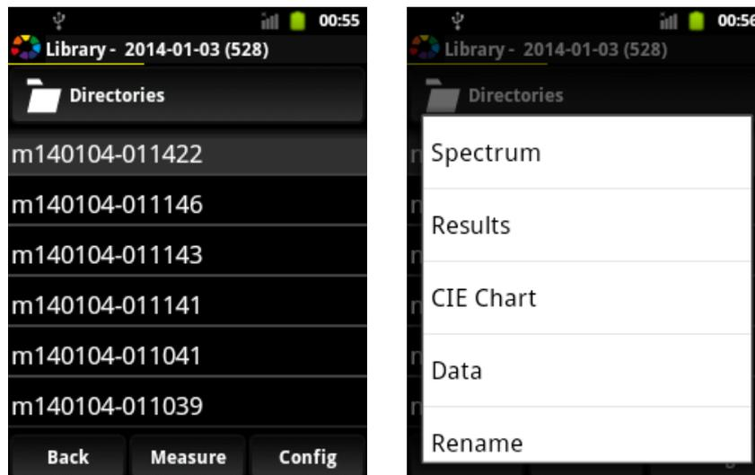
The Library screen shows measurements in the current directory and allows selecting the measurement which is displayed on the presentation screens. After a selection is made (by tapping the desired line), the measurement is displayed on the spectrum screen and is set as the current one. Any measurement taken is automatically set as the current measurement.
