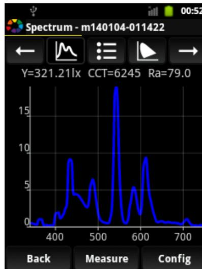
The Spectrum screen presents the spectrum chart of a measurement with several parameters at the top. The name of the measurement being presented is always shown in the title bar next to the GOSSEN icon.
