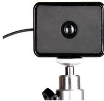
The set includes an optical measuring probe, fiber optics and adaptor for the mini-spectrometer with a coder for automatic detection of accessory calibration file. The measuring probe can be installed on a tripod for distance measurements. Alternatively, it can be hanged directly on a screen with the use of a special stripe for contact measurements.
