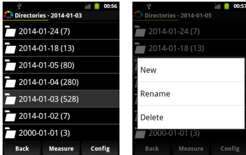
The directories screen shows directories in which the measurement results are stored. It also provides you with any easy tool to manage them. They are created automatically on the micro SD card where the measurements are collected and named using the date on which they were taken. You can manage directories using the **context menu**.
