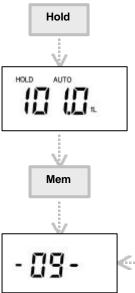
The measurement value to be memorized is locked by the Hold key in the display. By pressing the key Mem you will enter the value to be stored in the next free memory location. An acoustic signal confirms "value stored in memory".
