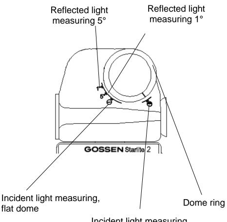
Incident light measuring, spherical dome
