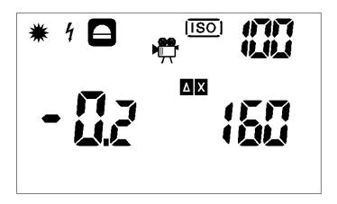
A shutter angle other than 180° has a direct influence on all measuring functions in the CINE function; corrected measuring values are shown directly in the display.
