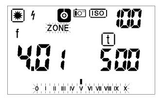
6 Measuring functions- Flash light 1 In essence, flash measuring can be carried out in all diffuser settings (incident or reflected light measuring modes). Furthermore, flashes can be measured with or without a sync cord (cord/noncord). If a sync cord is used, the flash is automatically triggered and measured with the measuring button M.
