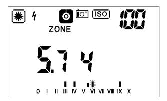
If, by mistake, you take a zone measurement in the incident light mode (flat or spherical diffuser), you are reminded by the flashing diffusor symbol that you have to set the diffuser ring to 1 ° spot metering.
