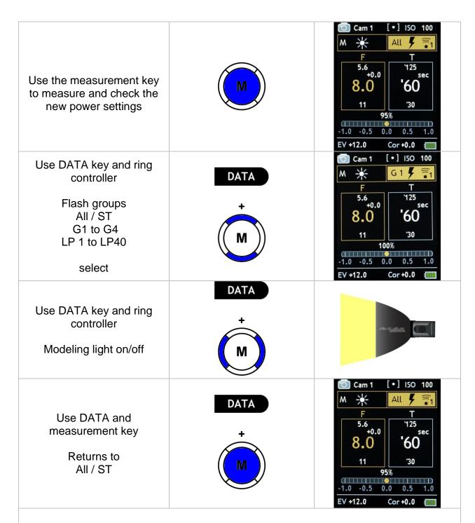
After measuring and setting all groups you can step through the values of the separate groups by using the DATA key and ring controller.
