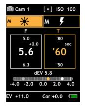
The average, minimum and maximum values can be displayed one after the other by pressing the data key.
