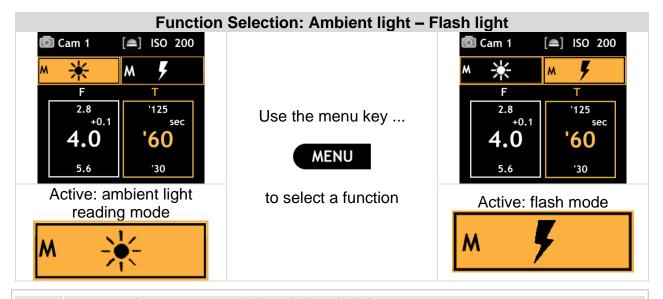
Measured f-stop increments (1 EV, 1/2 EV, 1/3 EV) can be adapted as required by the user in Menu – User (Cam 1, Cam 2, Cam 3, Cine) - EV Steps (see page 27).
